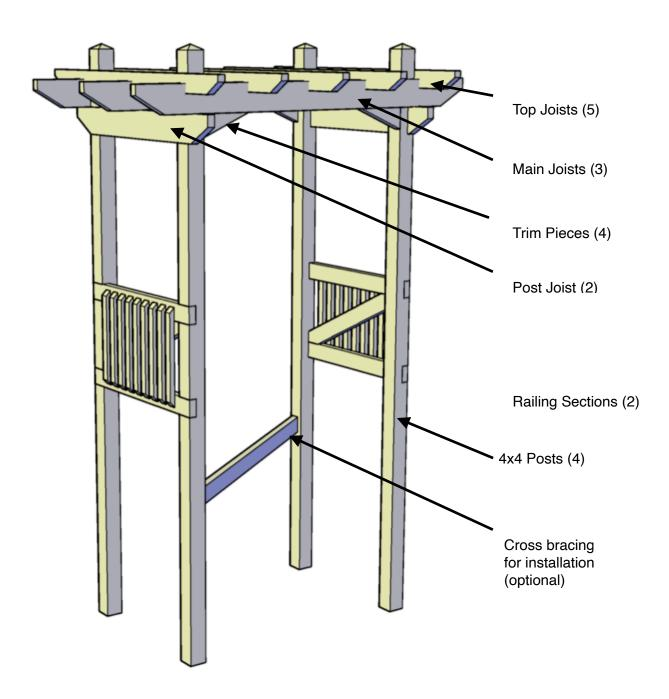
Note: \* Each post consists of two shiplap (L-notched) post halves (not shown) to be assembled on site.
